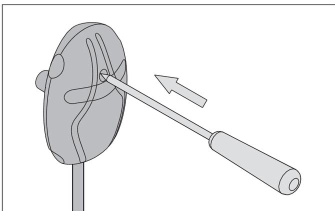
**Figure 9. Reset button for overheat protector**
