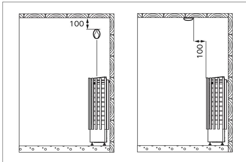
**Figure 6. Installing the sensor (all dimensions in millimeters)**
