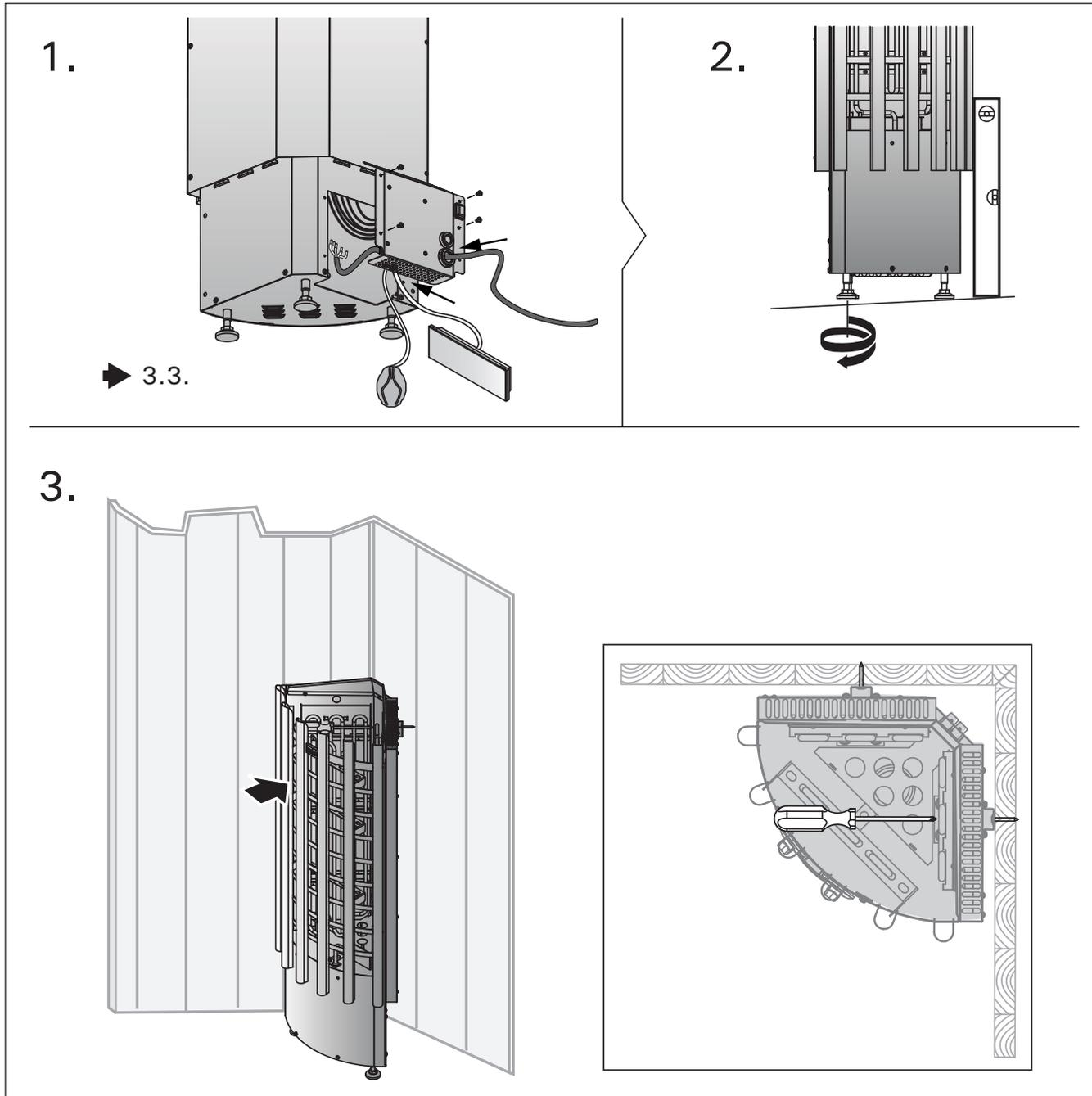
**Figure 8. Installing the heater**
