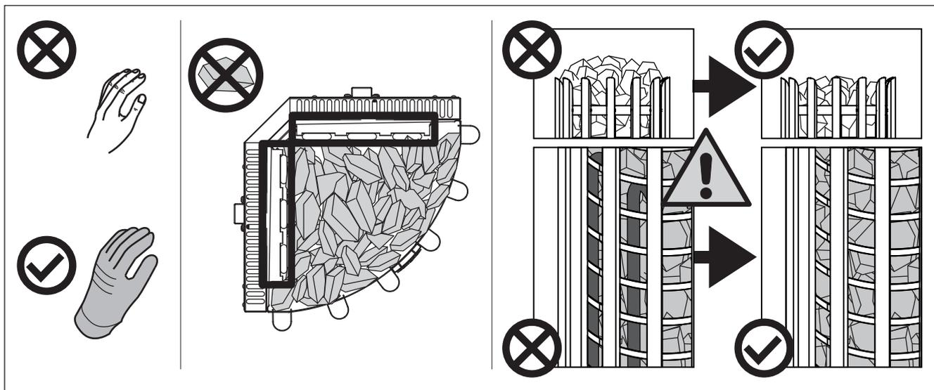
Figure 1. Piling of the sauna stones
