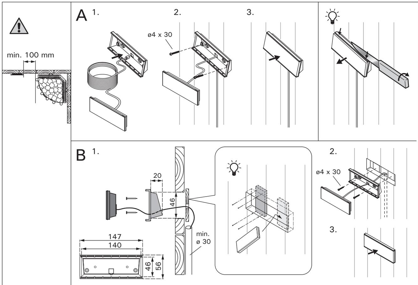
**Figure 7. Installing the control panel (all dimensions in millimeters)**
