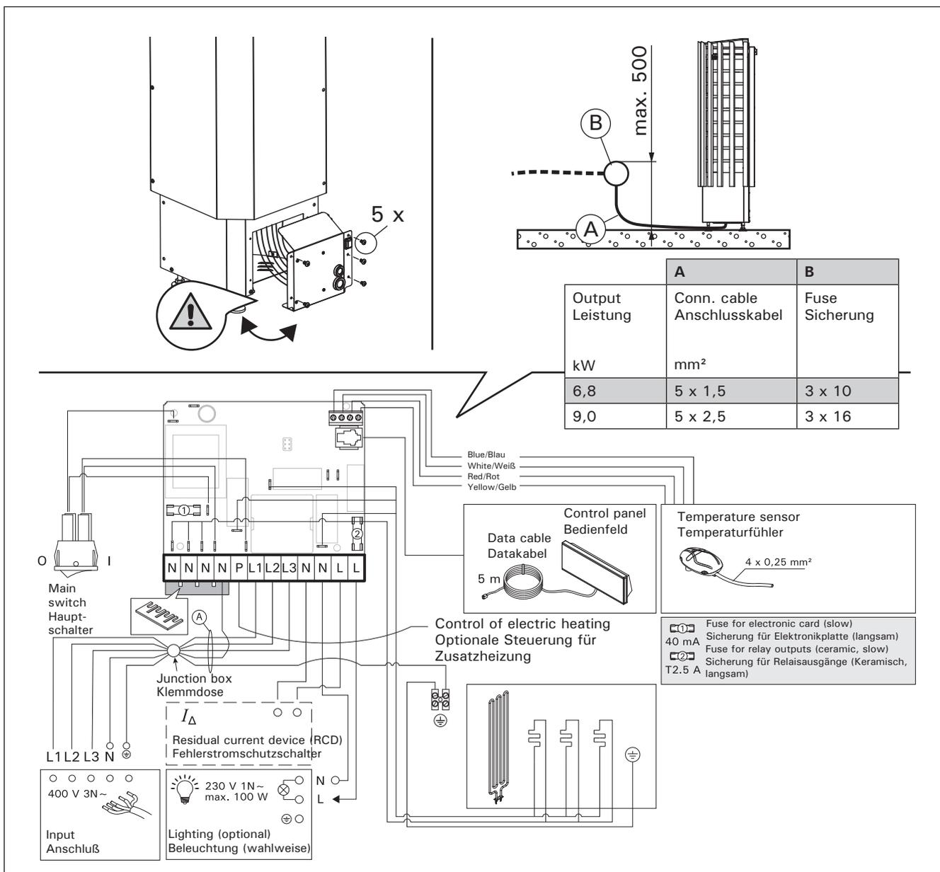
Figure 5. Electrical connections
