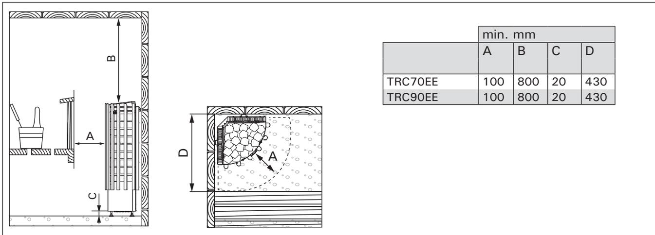
Figure 4. Safety distances (all dimensions in millimeters)
